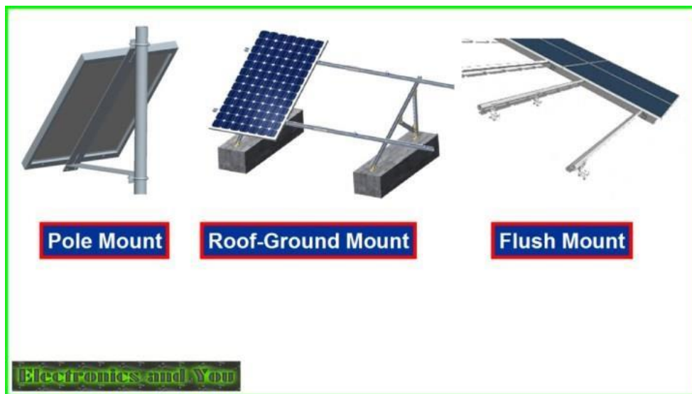
Fig 2.10 Different mounting structure
