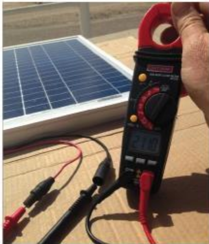
Figure 1.35 : digital clamp-on ammeter with leads is used to perform the circuit measurements.
