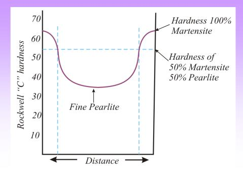
Typical hardness test survey made along a diameter of a quenched cylinder
