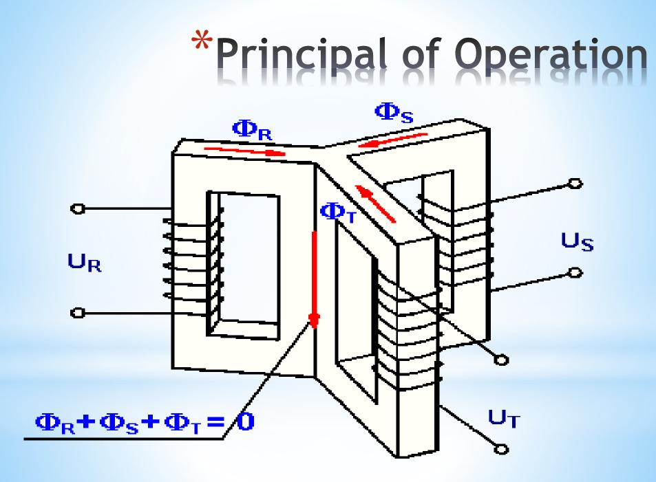
\*The three cores are arrange at 120° from each other. Only primary windings are shown on the cores for simplicity.
