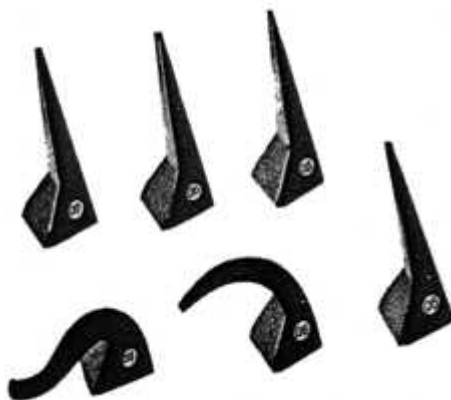
Figure 5.4 Self Supporting Cones prior to firing (top) and after (bottom)
