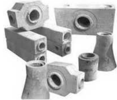
Fig 1.2: Different shapes of refractories for lining
